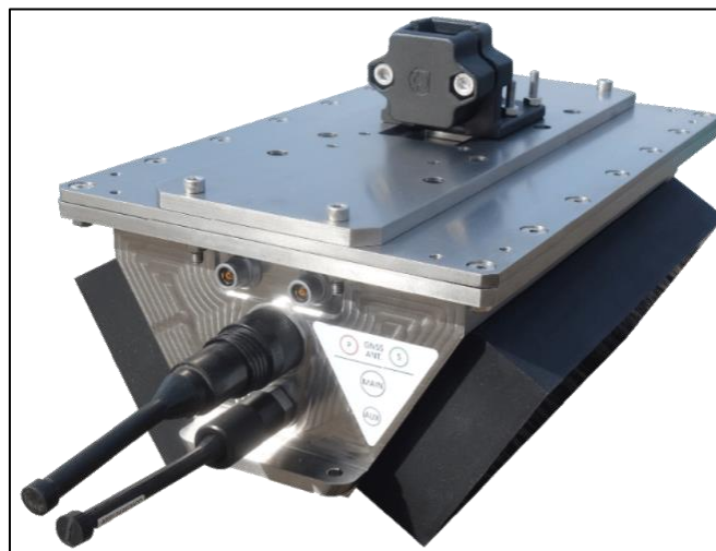
Figure 8 Bathyswath-3 Alpha mounted with 250kHz transducers
