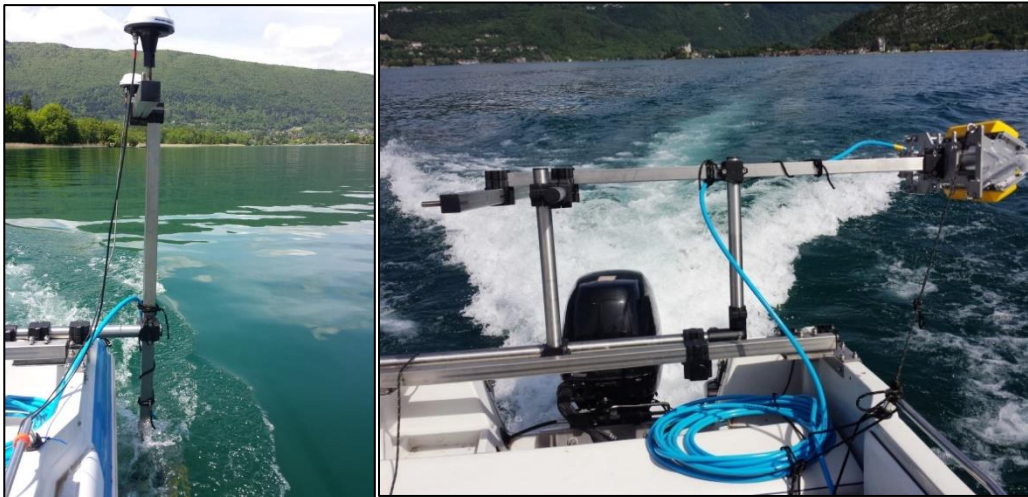
Figure 18_Bathyswath-2-UW side installation
