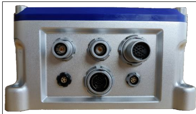
Figure 11 NAVBOX connectors side view
