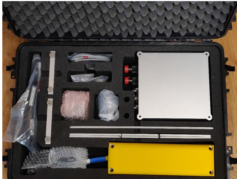
Figure 24 Transit suitcase with Bathyswath-2 Omega + 234kHz transducers
