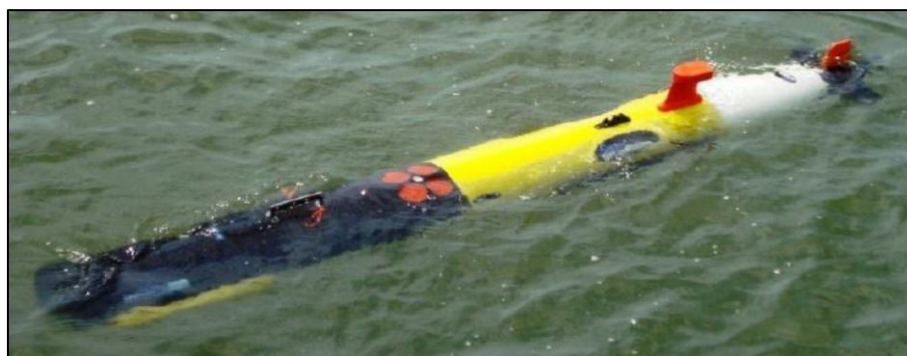
Figure 8_Bathyswath on Remus AUV
