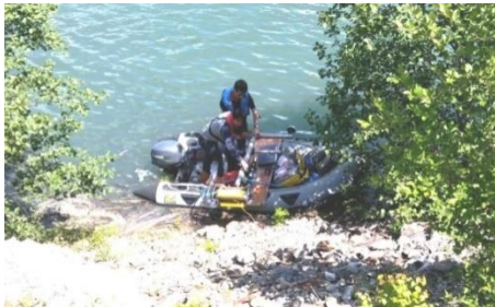
Figure 12 Setting up Bathyswath sonar on a RIB
